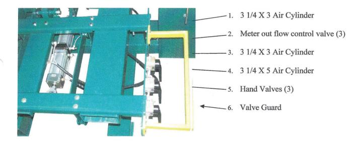
Smart Products BLOCK PALLET PREP Blade Tensioning System
